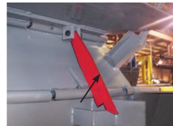
Latch Position (Illustrated in red for clarity)
